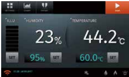
7" Full Touch Screen TFT LCD (Smart-Lab™ Controller)
