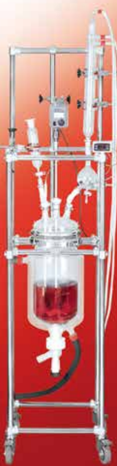
0.5~20 Lit. Suspended-Model III Double-Wall Vessel Good for Economic Operation
