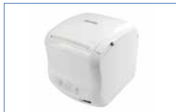
(1) RS-232C Thermal Printer, "WBA-100"
