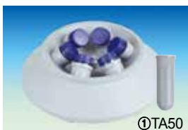
(1) Fixed Angle Rotor ; 50ml 6Holes, “R5006”
