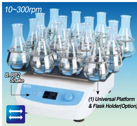
Figure ; Orbital Shaker “MaXshake™ RP2” + (1) Universal Platform & Flask Holder(Optional)
