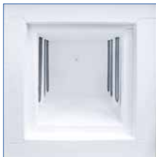
Inner Chamber of Exposed Heating Elements-type
