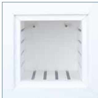
Inner Chamber of Exposed Heating Elements-type
