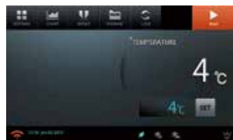
7" Full Touch Screen TFT LCD (Smart-Lab™ Controller)
