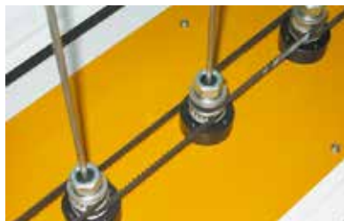
Geared DC Motor with Special Timing Belt
