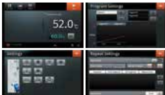
4” Full Touch Screen TFT LCD (Smart-Lab™ Controller)
