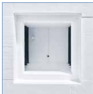
Inner Chamber of Exposed Heating Elements-type
