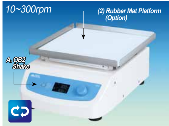
Figure ; Orbital Shaker “MaXshake™ OB2” + (2) Rubber Mat Platform(Optional)
