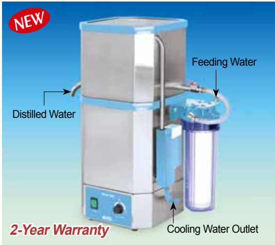
3.5 & 7.5 Lit/hr Cabinet-type Water Still “CWS”
