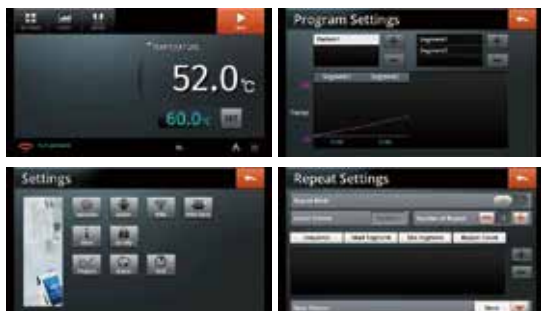
4" Full Touch Screen TFT LCD (Smart-Lab™ Controller)
