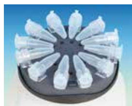
(3) Microtube Platform Head, 0.5~2.0ml Tube "PM310" (Optional)
